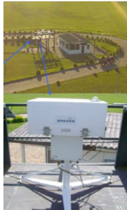
Figure 20 – Southern Space Observatory Building and Brewer Spectrophotometer MKIII #167.
